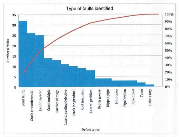
Figure 1: Numbers and percentages of fault types
