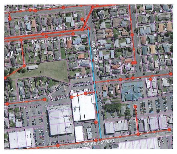
Figure 1 Logan Street Wastewater main renewal site (Subject pipes highlighted in cyan)
