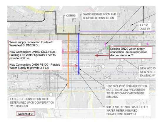
The WWL modelling team have indicated that there is 75-80 m of pressure in the water supply network at the point connection into the DN200 DI Wakefield Street watermain. This modelling result is based on a 2018 model which does not factor in future and proposed and developments. The applicant has advised a fire demand of 52.6 L/s and a domestic flow of 3.1 L/s. Calculations are required to support the assessment and demonstrate that this can be achieved from the public network.
