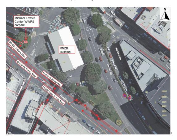
The applicant indicates that there is an existing WW service lateral which services the RNZB building (DN unknown). The applicant's drawing suggests that this service lateral connects directly in to the existing DN350 CI Rising main on Wakefield Street although, their reporting and labels indicate they have mistaken this to the DN450 Gravity main.
