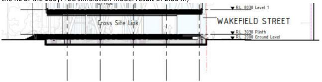
The applicant has provided freeboard to the top of slab (as opposed to underside of slab as typically required by WWL). The applicant has stated that this has been agreed with WCC BC team on the basis of that:
