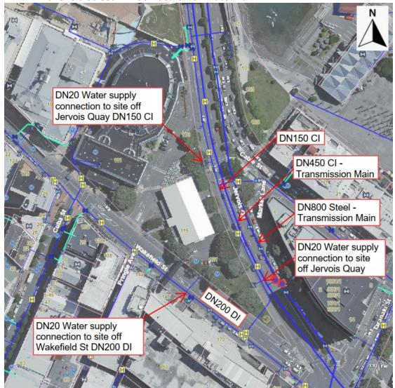
The applicant claims there is an existing DN40 water supply from the DN200 DI Wakefield watermain which services the existing Royal NZ Ballet building. This service is not shown on Council Records nor are As-Built records provided to prove this connection.
