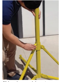
Slide pole up and down to adjust height then release pin to lock in place
