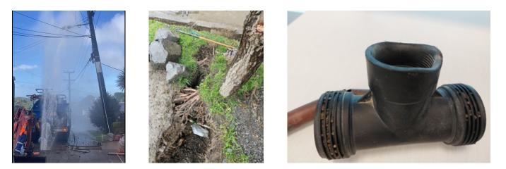
Service connections are the pipework, fittings and tobies that connect council's water pipes to residential and commercial properties. Like other water infrastructure across the region, these are getting old and deteriorating, causing leaks which can result in significant water loss.
