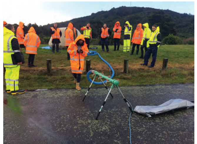
The tap stand and hoses attaching it to the bladder. This would be set up in the street or in a community emergency hub for members of the community to collect their daily water allowance.
