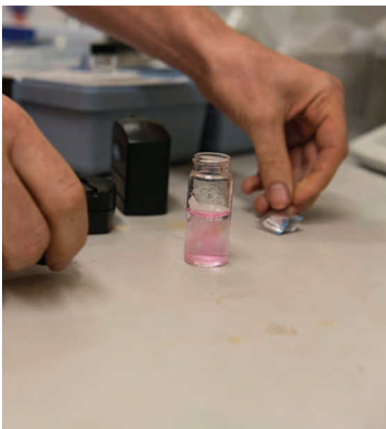
Drinking water testing to check residual chlorine levels.
