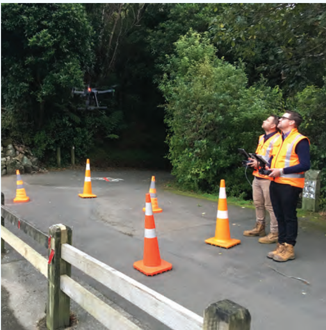
The drone is operated by a crew of two – one person flying the drone and the other capturing the images. The drone is typically flying about 40 metres high (vertically) with images taken roughly every 10 metres (horizontally).
