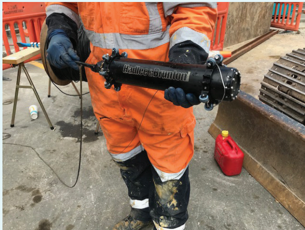
The new CCTV camera developed for the sludge pipes under Mt Albert.
