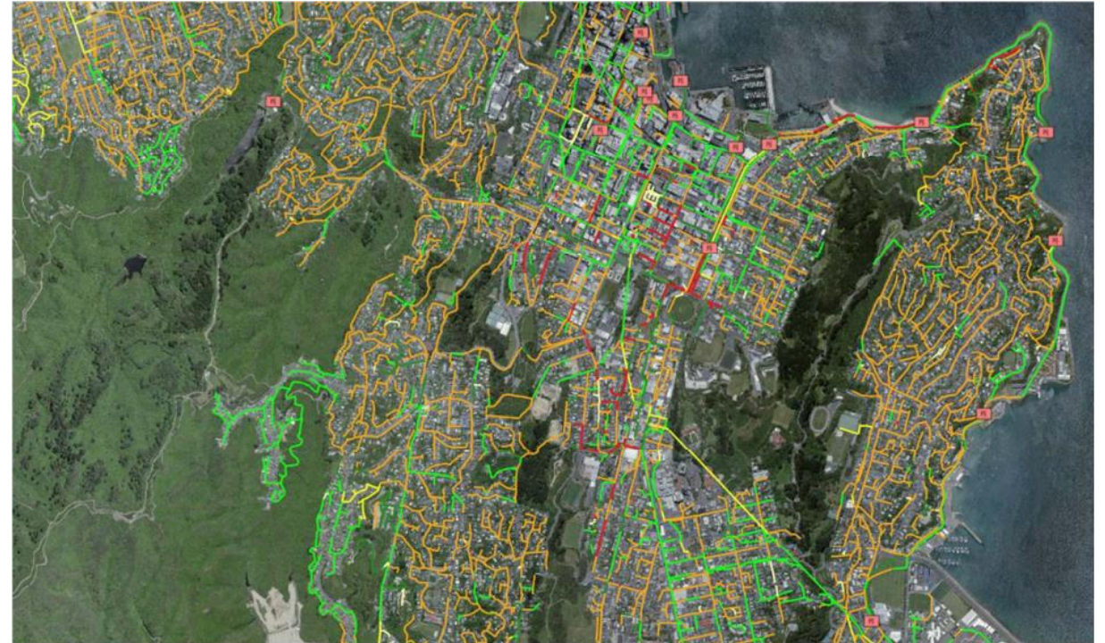
Wellington Central North and West: Wastewater Condition
