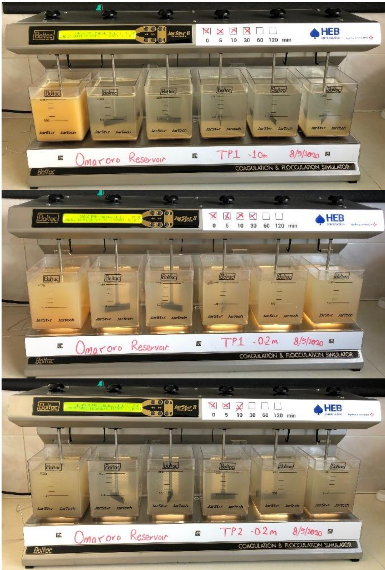
Photo 10 Bench testing results after 30 minutes settling
