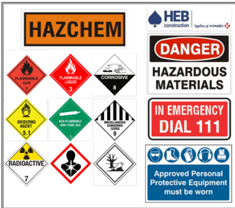
Figure 8: Hazardous Substances Warning Signs to be used on site.
