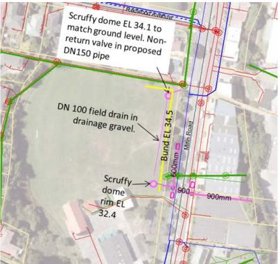
Figure 4. Wellington Water's Option 2: Bund on east side of field in addition to proposed assets in Option 1
