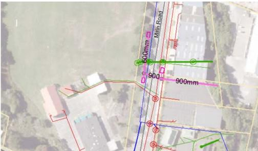
Figure 3. Wellington Water's Option 1: High-capacity sumps and new outfall pipe only
