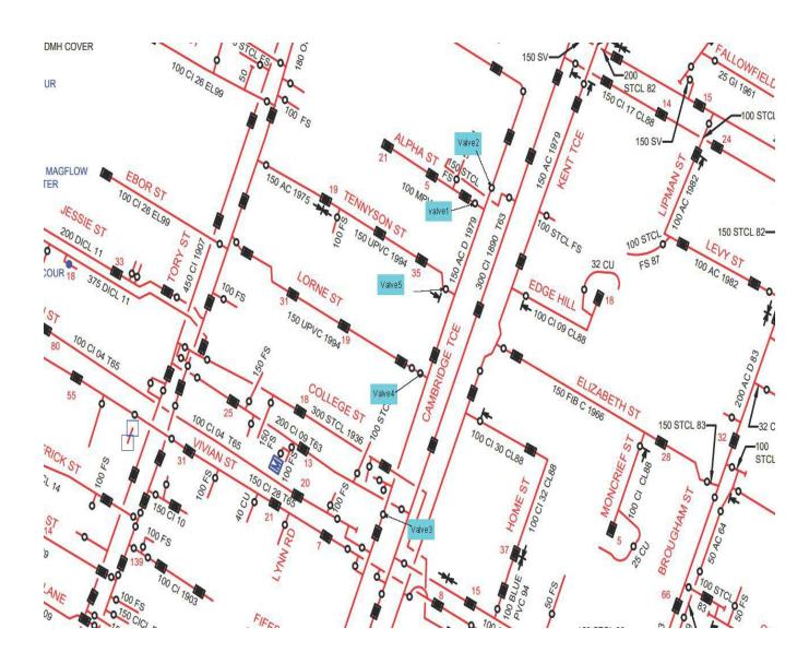
As this section of watermain can be isolated vie 1 Sluice valve(SV1), The only risk that could disrupt further customers is if SV 1 fails and the works cannot be carried out with the influx of water. The connection point is labelled as MPVC which could be worked on with a small quantity. If this occurs and we are unable to achieve the connection, further valves will be closed and disrupt addition Wellington Water customers.
