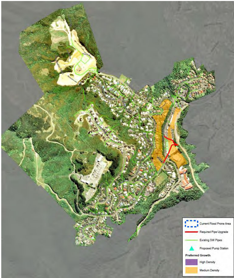
Figure 17 –Potential stormwater upgrades for Crofton Downs
