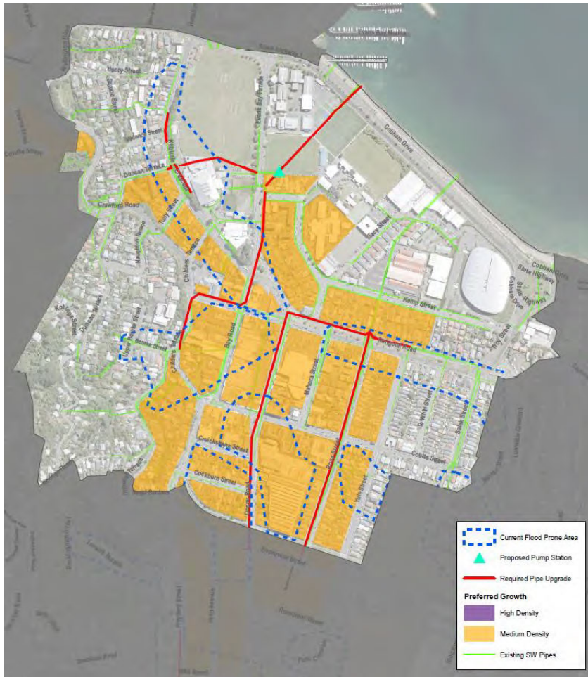
Figure 40 – Predicted flooding and potential stormwater upgrades for Kilbirnie.
