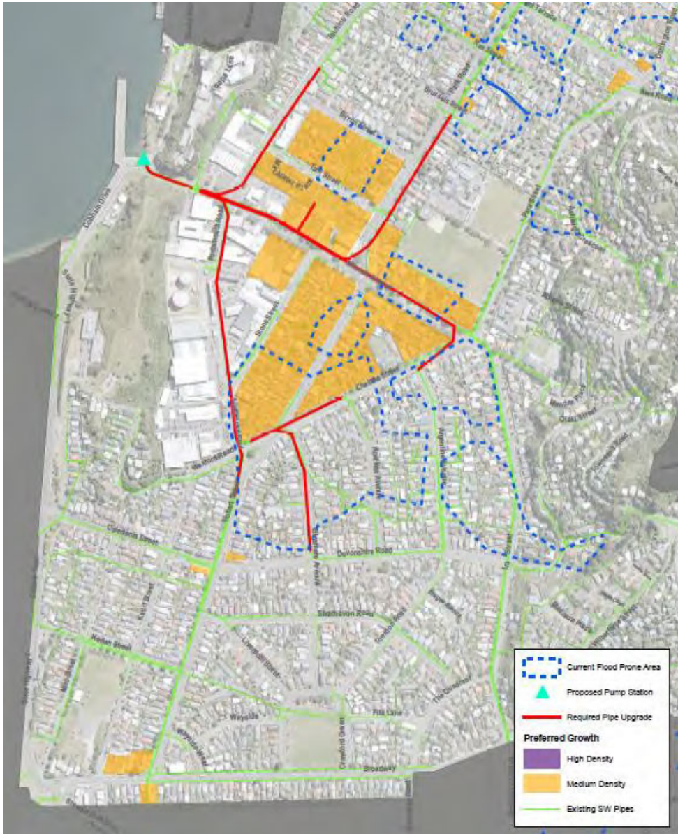
Figure 45 – Predicted flooding and potential stormwater upgrades for Miramar.
