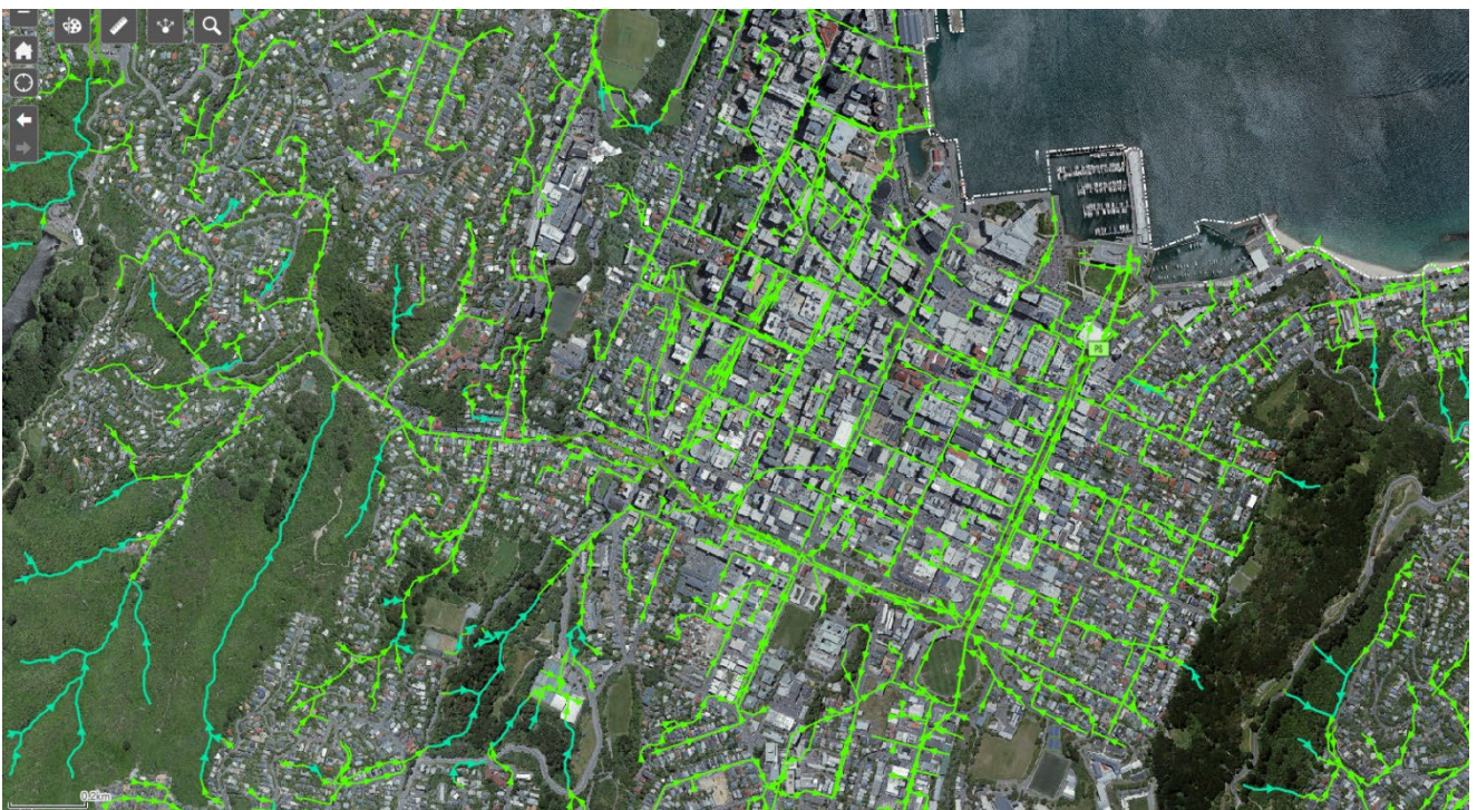
Figure 3-8: Wellington CBD streams are piped for most or all their length, except for some headwaters
