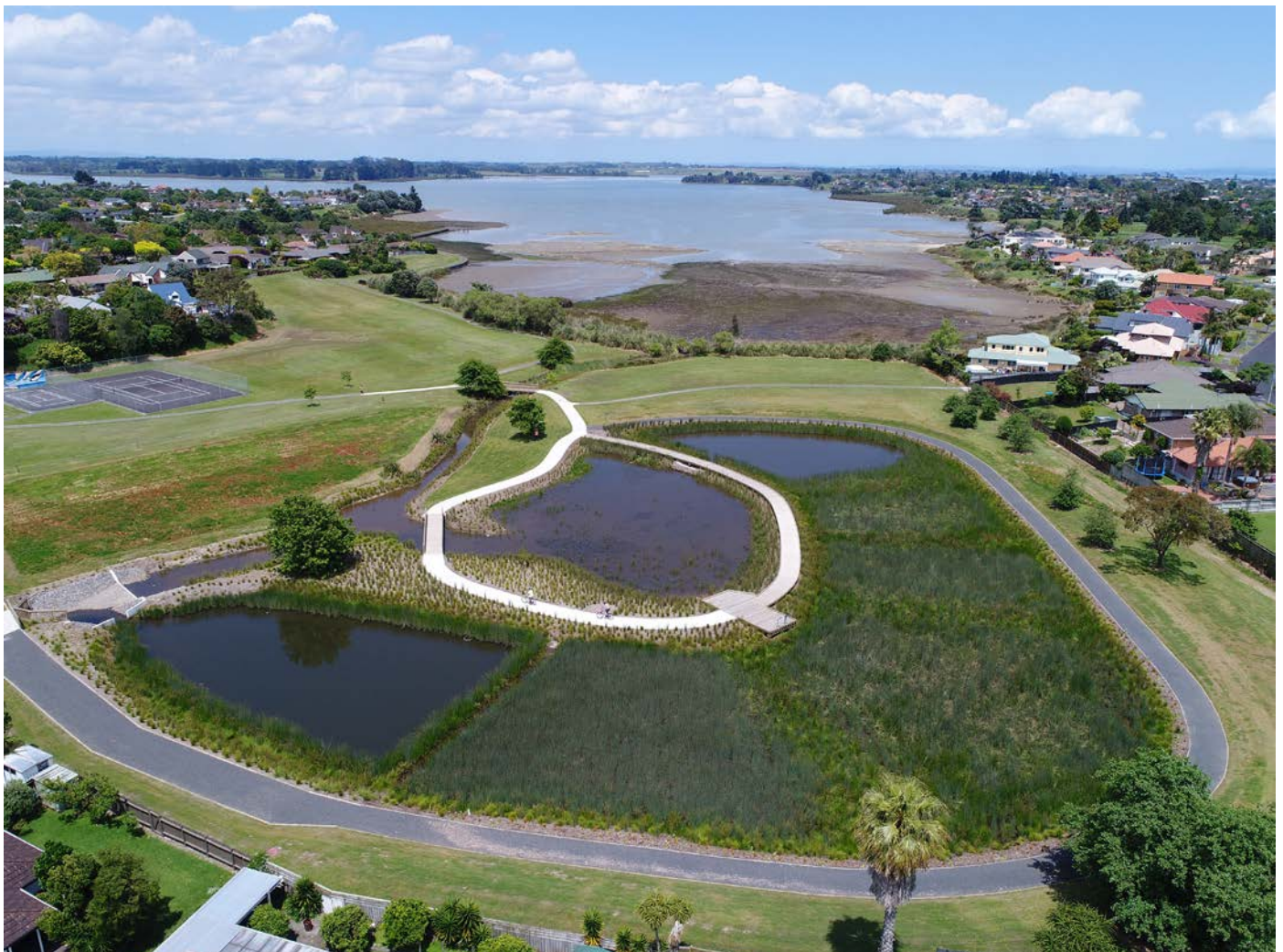
Figure 2: Example of recently planted constructed wetland integrated with public park and adjacent properties. Brylee Reserve, Auckland.
